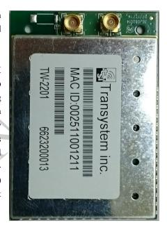
With the small footprint, low cost, and rich features set, TW-2201 Embedded WiFi module is well suited for Internet of Things (IoT) applications. The module is small enough to be added to most devices.
